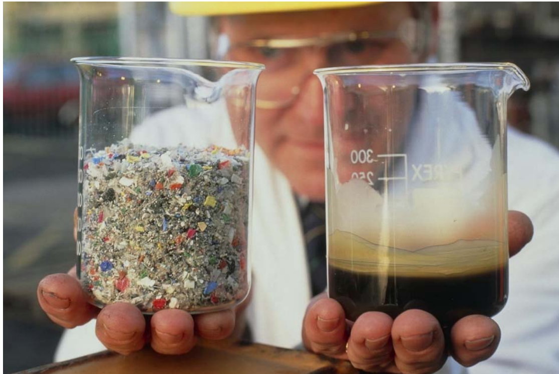
Chemical engineer David Wilson holding a sample of waste plastic (left) and oil reclaimed from it at BP's Feedstock Recycling Pilot Plant in Grangemouth, Scotland. James King-Holmes / Science Source
