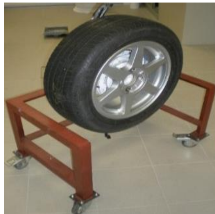
Figure 3 Unloaded condition tyre test setup
