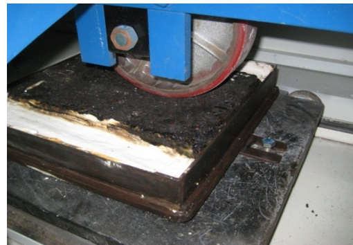
Fig. 13: Wheel tracking test
