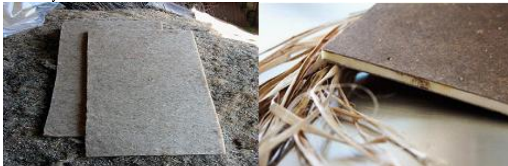
Fig.6. (a) Kenaf panels (KEFI Company). Fig.6. (b) Kenaf Insulated panel (Univ. of North Texas).
