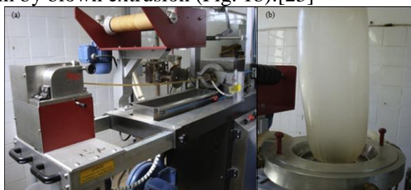
Fig.7: Film production by extrusion: (a) acquisition of pellets and (b) formation of tubular film.[23]
