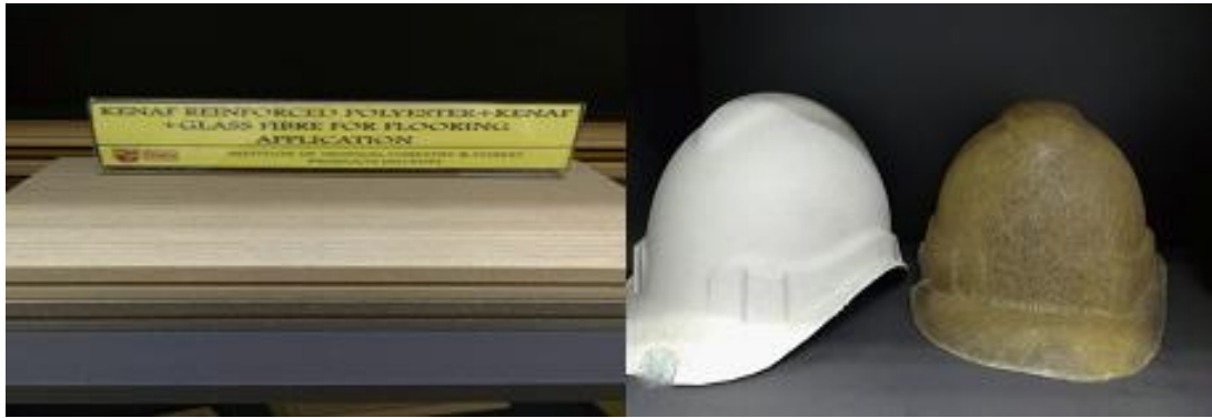
Fig.7. Flooring panel and helmet from Kenaf fibre reinforced polymer composites (INTROP-UPM).
