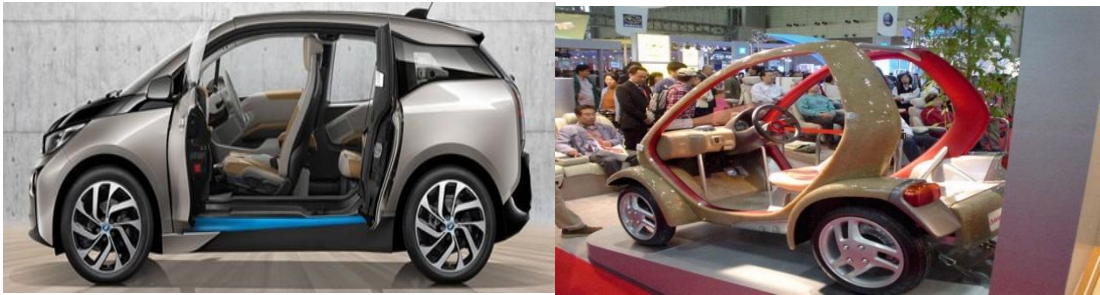
Fig.1. Car body of BMW i3 and Toyota made from Kenaf reinforced polymer composites.
