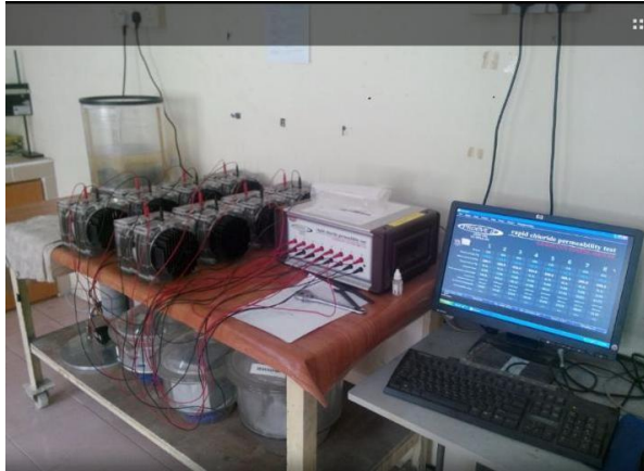
Fig.1.Rapid chloride permeability test (RCPT) setup
