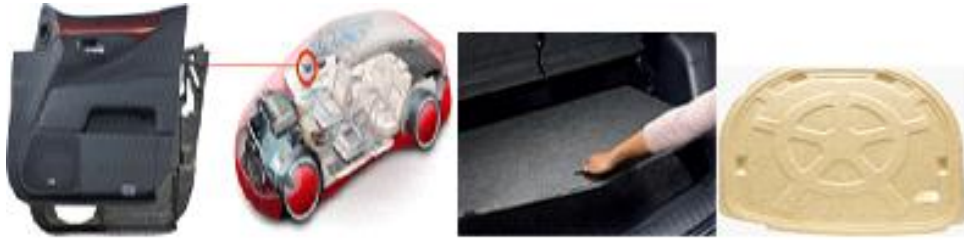
Fig.4. Door trim using kenaf base material
