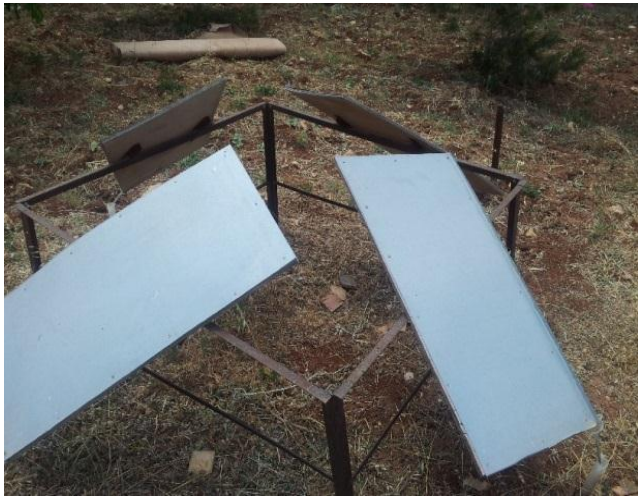
Figure (3): Dew water collector panels that used to collecting data in this research
