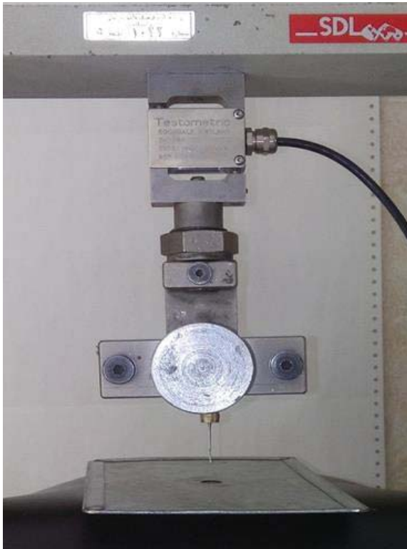
Fig. 2. A specimen under needle penetration test.
