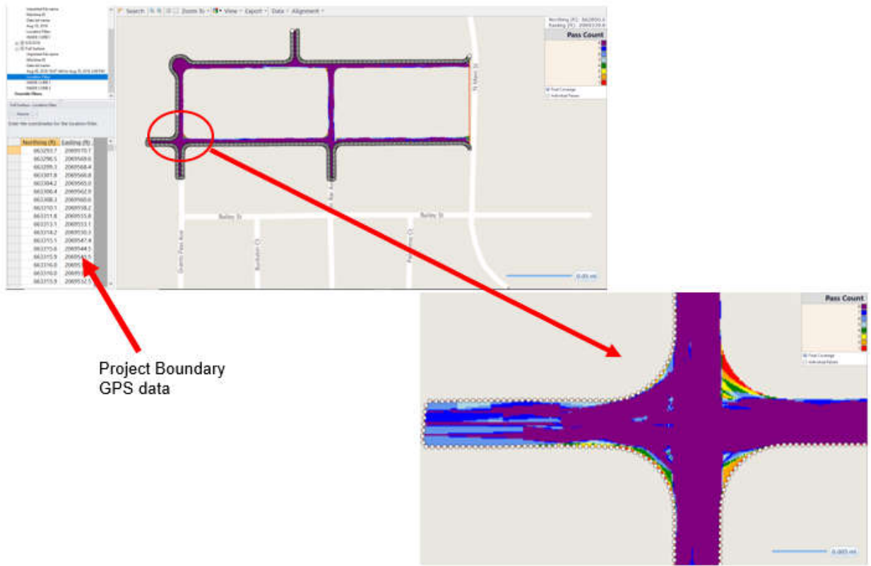
Figure 30 Filtering the IC Data Based on Road Boundary GPS Data
