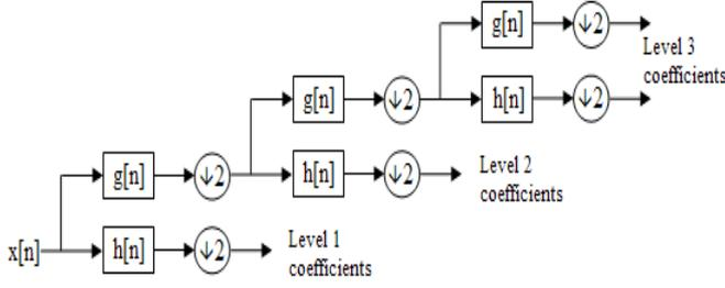
Figure 2. Three level of the discrete wavelet decomposition
