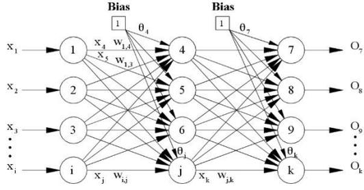
Figure3. A schematic diagram of a Multi-Layer Perceptron
