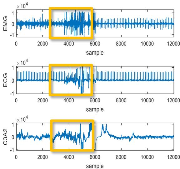
Figure 1. Presentation of the apnea disorder window in EMG, ECG, and EEG signals
