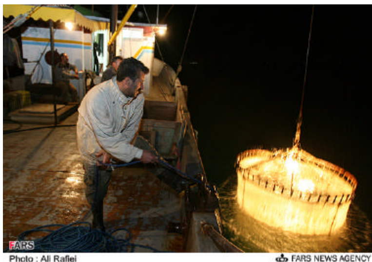
Fig. 8: View of Conical lift net (Kilka net). www.farsnews.com
