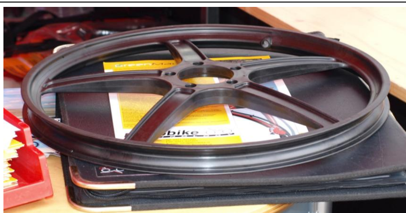
Picture 16 - Composite 406 mm wheel for velomobiles
