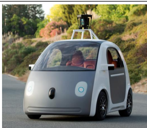
Picture 18 – Google self-driving vehicle prototype with no steering wheel or pedals
