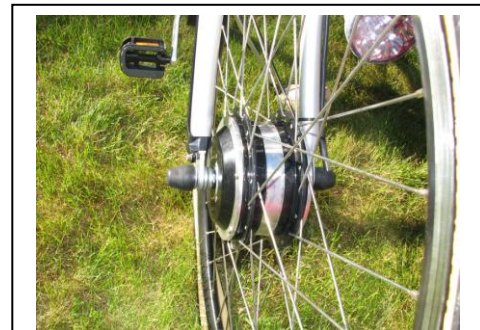
Picture 8- Geared front motor installed on bicycle
