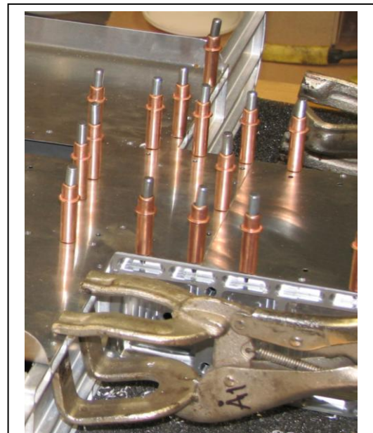
Picture 14 - Typical blind nuts assembly technique using clecos, vices
