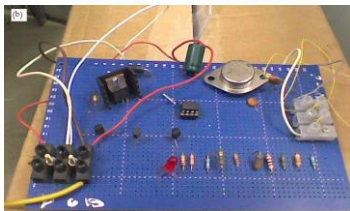
Fig. 6 The implemented charge controller circuit on a stripboard.
