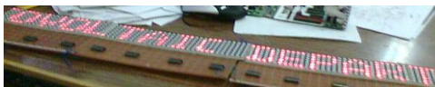
Fig. 14 The moving message display for 22 characters with spacing (27 Dot-matrices) after moving some characters.
