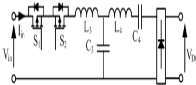
Chang-Ya Huang [3] designed a multi-path pick up controller as shown in Fig 5, which was able to control the mutual inductance between the cores. This topology achieved efficiency of 96% at 2 KW output, and provided above 90% for all power ranges. In addition, it worked by controlling the number of active LCL networks based on the induced voltage in the secondary, and then the power could be regulated between the coils, as shown in the following equation.
