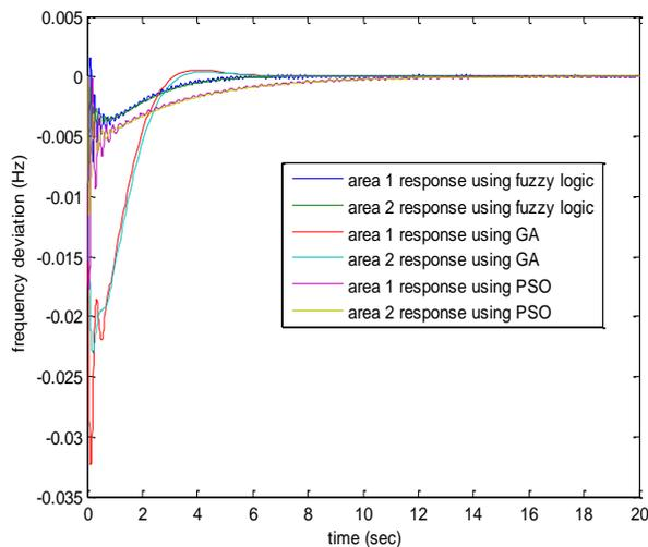
Figure (19): Frequency Deviation Responses Of Two Power System Areas In Case of GA, PSO and Fuzzy PID Tuning
