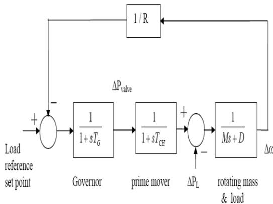
Figure 2. Block Diagram of Primary LFC Loop for Single Area System
