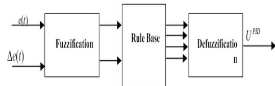
Figure 10 Fuzzy Logic Control Structure
