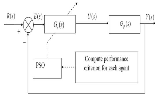
Figure 15 PID tuning using PSO algorithm
