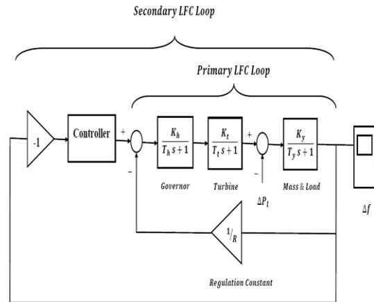
Figure 3. Block diagram of single area system with a controller
