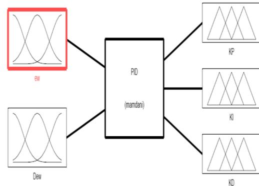
Figure 9 Fuzzy Logic Model Input - Outputs
