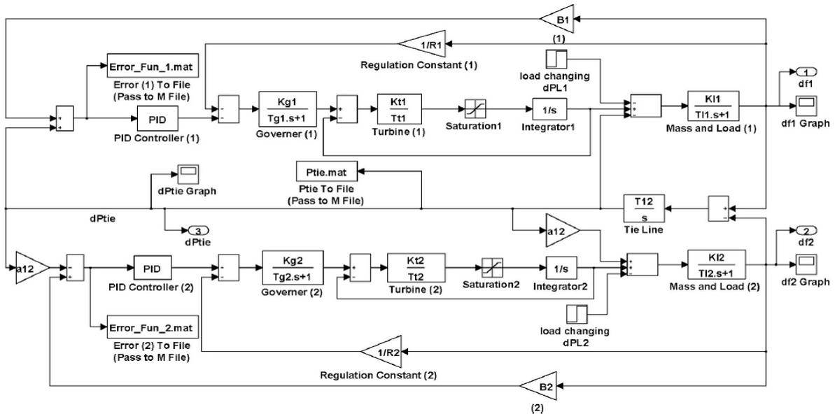
Figure (5): The Non-Linearized Two-Area Power System Simulink Model with Genetic Algorithm-Tuned PID Controller
