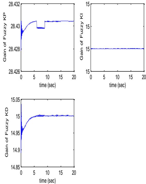
Figure (18): Gains of PID Tuned Using Fuzzy Algorithm for two different area power system
