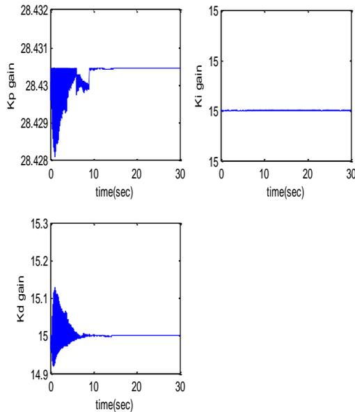
Figure (16): Gains of PID Tuned Using Fuzzy Algorithm for single area power system
