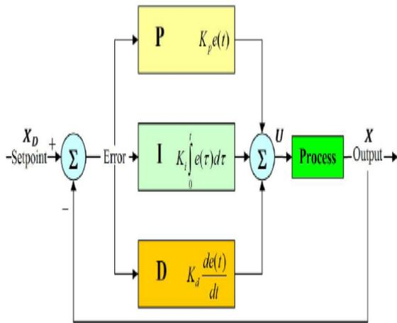
Figure 6 Schematic of the PID Controller – Non Interacting Form
