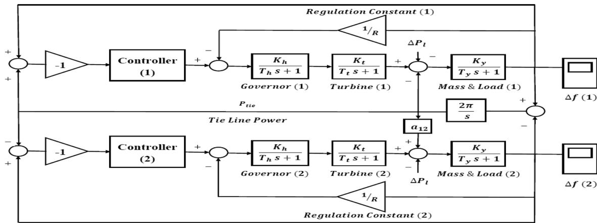
Figure (4). Block Diagram Of Interconnected Areas
