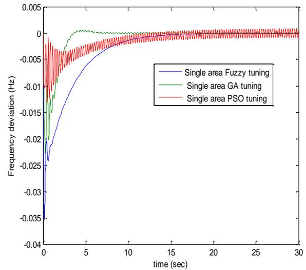
Figure (17): Frequency Deviation Responses Of single area Power System In Case of GA , PSO and Fuzzy PID Tuning
