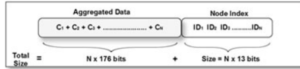
Figure 4. An illustration of the aggregated data at the cluster head. N is the number of nodes in the cluster. The package consists of the encrypted data and the node IDs.
