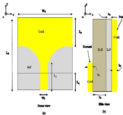
Figure 1 : Geometry and configuration of the proposed Antenna
