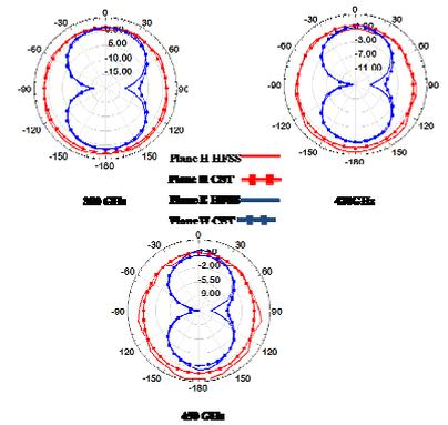
Figure3: Simulated 2D polar radiation patterns of the proposed terahertz antenna at several frequencies on both the E- and H-planes by CST and HFSS simulators.
