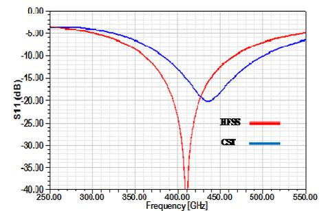
Figure 2: Simulated S11 of the proposed antenna using CST and HFSS software.
