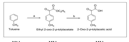
M1d M2d M3d Reagents and conditions: (a) CHCl<sub>3</sub>, ethoxyl chloride, 0-5 <sup>0</sup>C, 40 min, then AlCl<sub>3</sub>, 0-5<sup>0</sup>C, 80 min (b) MeOH, 4N NaOH, 40 min, 1N HCl
