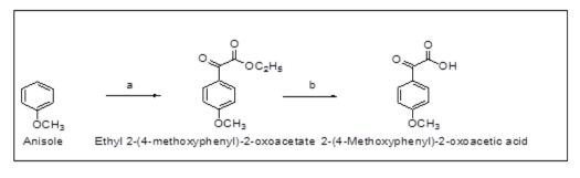
$\begin{array}{ccc} M1c & M2c & M3c \\ \mbox{Reagents and conditions:} & (a) CHCl_3, ethoxyl chloride, 0-5 \ ^0C, 40 \ min, then \ AlCl_3, 0-5^0 \ C, 80 \ min \\ & (b) \ MeOH, 4N \ NaOH, 40 \ min, 1N \ HCl \end{array}$
