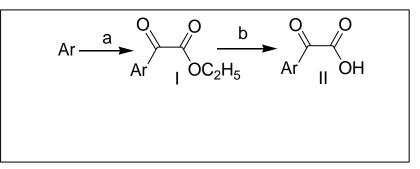
**Reagents and conditions:** (a) CHCl<sub>3</sub>, ethoxyl chloride, 0-5 <sup>0</sup>C,40 min, then AlCl<sub>3</sub>, 0-5 <sup>0</sup>C, 80 min (b) MeOH, 4N NaOH, 40 min, 1N HCl.
