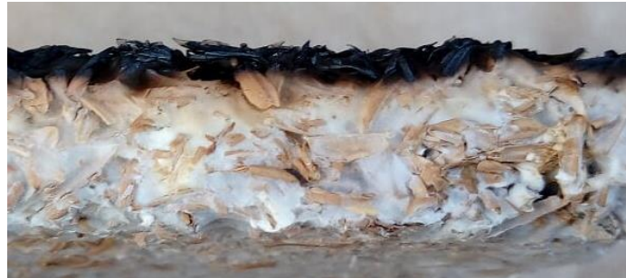
Figure 3: Char formation on the exposed surface.
