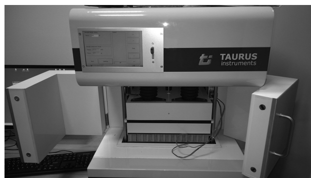
Figure 3 The TLP 300 DTX-1 thermal conductivity measuring device.
