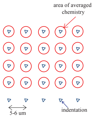
Figure 4-8: A schematic showing a 5 \times 5 indentation grids. Blue triangles depict indentation impressions obtained indenting with a Berkovich tip. The spacing between indentations varies depending on P_{max} and maturity of the formations; 5 \mu\text{m} -spacing and 6 \mu\text{m} -spacing were used indenting mature and immature formations, respectively, with P_{max} = 4.8\text{mN} . Red circles simulate 1\mu\text{m} -radius areas around indentation tests where x-ray intensities are averaged. The triangles, triangle spacing, and circles areas are not drawn to scale.
