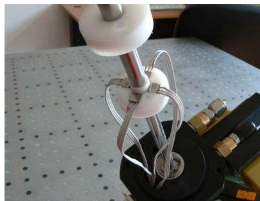
Fig. 23. Teflon ring used to mount the microphones flush with the tube wall.
