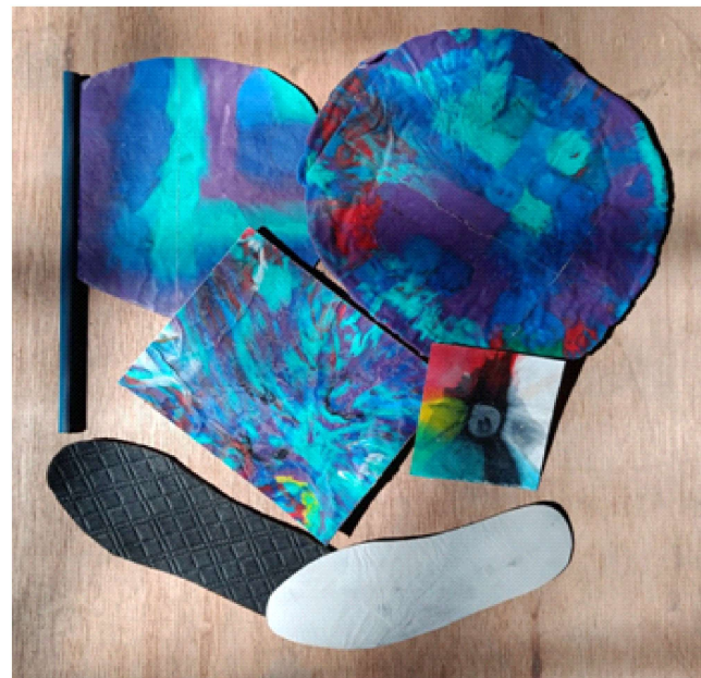
Figure 3.4 : Plastic Lumber, Shoe insole, Plastic Coasters and Plastic Hand Fan PET bottle sheds after compression
