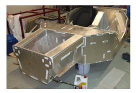
Figure 3: FEA and final chassis assembly
