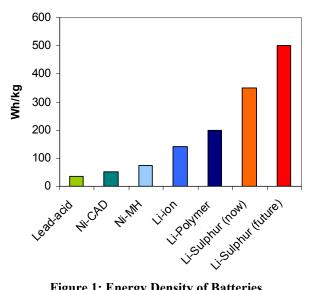
**Figure 1: Energy Density of Batteries**
