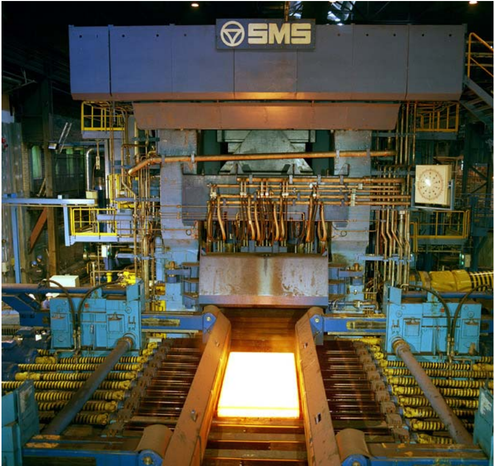
Figure 4. Rolling in the heavy plate mill in Oxelösund.
