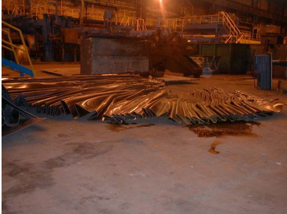
Figure 7. A thin plate after buckling and breakdown.
