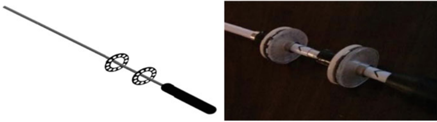
Fig. 2 A prototype of an ablation probe with two LED rings
