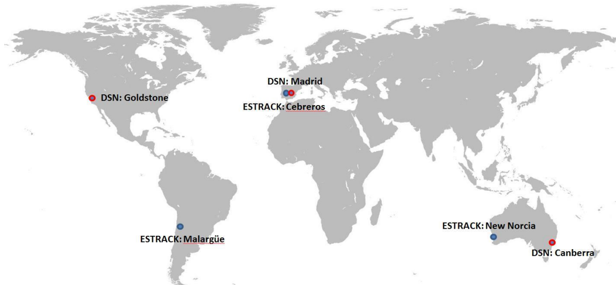
Figure 2. Rosetta ground station facilities around the globe. Rosetta dumps the mission data mainly through the ESA-ESTRACK Deep Space Antennas (DSA, in blue), with important support from NASA Deep Space Network (DSN, in red). Their distributed location around the globe ensure a ~24h coverage.
