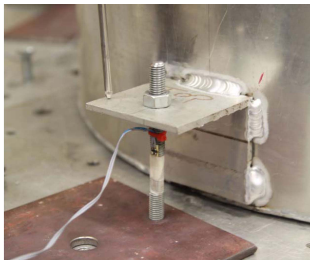
Fig. 6 Anchor bolt used to fix the tank to the shake table
