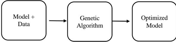
Figure 2: Genetic algorithm with  $l_1$  distance cost function is used in optimizing the model. The GA makes use of population type bit string, crossover ratio of 0.8, constraint tolerance of  $10^{-6}$ , and function tolerance of  $10^{-4}$ . Elitist method (MATLAB 2014 optimization toolbox) was used for selection.
