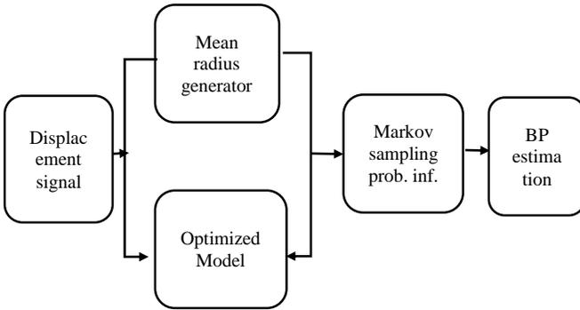
Figure 3: The complete algorithm for BP estimation. The displacement signal is feed into the optimized model and mean radius generator which gives out a set of probable values for the blood pressure for the sampled set of parameters (E and h). This estimate is then feed into the probabilistic inference set up to determine the maximum likely BP.
