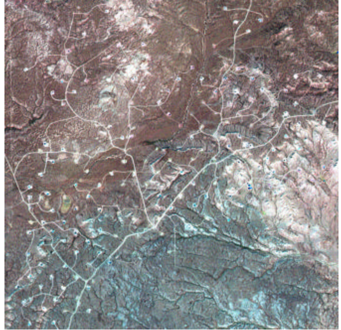
Figure 4. The Jonah Gas Field in 1999 after one year of full-field development at 80-acre spacing (8 well pads per square mile) using state-of-the-art drilling technology. The web of wells pads, access roads, compressor stations and waste pits is clearly visible. (Credit: Amos 2003).
