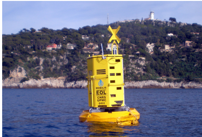
Figure 1 View of the EOL (Environnement Observable Littoral, CNRS-Mobilis) buoy deployed in the Bay of Villefranche sur Mer (France). The water column depth at this location is about 100 m.
