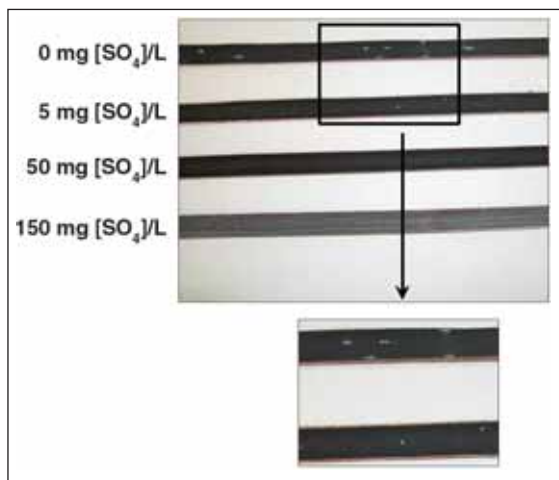
The interior surfaces of copper pipes exposed to 0, 5, 50, and 150 mg/L \text{SO}_4 at pH 9 (experimental runs 9–12) show pipe surface scales. A close-up image highlights the randomly dispersed blue-green corrosion by-product.
