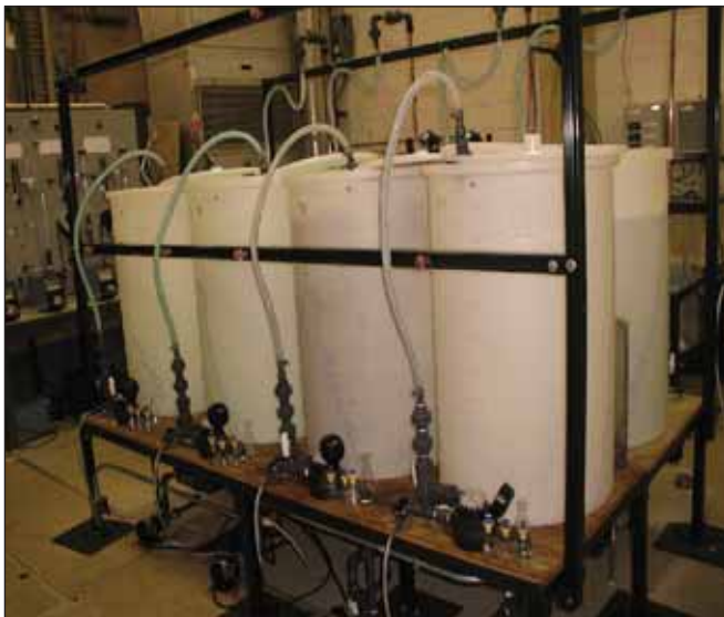
The pilot-scale copper recirculation system used in these experiments included 200-L (53-gal) heavy-duty polyethylene tanks.
