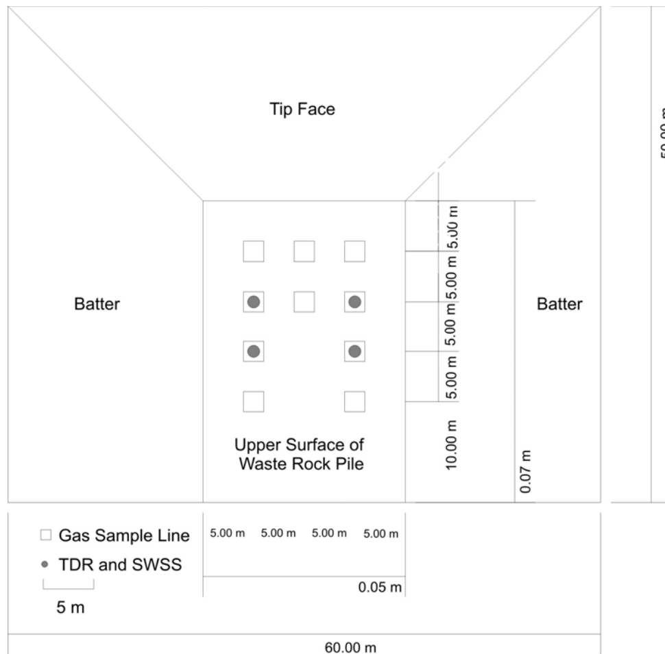
Figure 10. Aerial view of waste rock pile showing locations of instrumentation along the tip faces (TDR = time domain reflectance probes and SWSS = soil water suction sampler).
