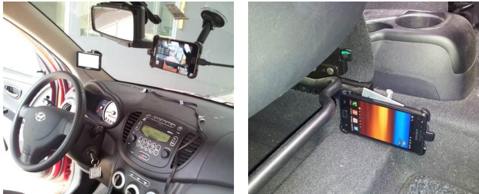
Figure 3: Smartphone-based data acquisition with one phone mounted on the windshield to record GPS and video (left) and a second one fixed on the front passenger seat to measure 3D acceleration (right)
