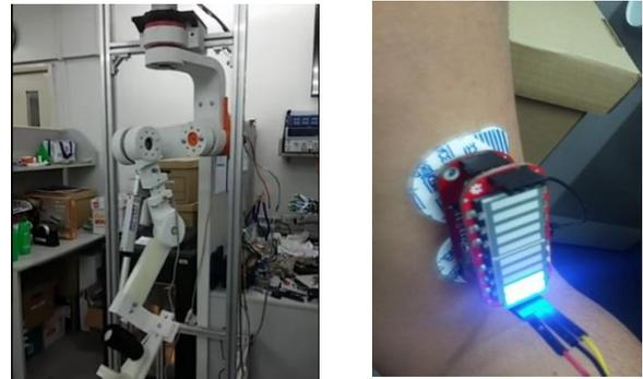
Figure 2. Agapay 5 -DOF Exoskeleton (Left) Myoware Sensor (Right)
