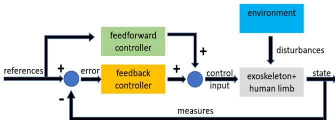
Figure 1. General control scheme. A feedback control calculates error from current state, and a feedforward control containing desired values are combined as a single control to trigger actuators. Environment acts like a disturbance affecting performance of the exoskeleton<sup>7</sup>.
