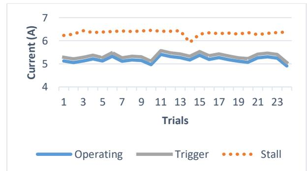
Figure 4. Stall condition characteristics at 5 A operating current
