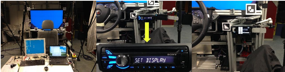
Figure 1 Experimental setup (a) complete (b) driver space and radio (c) smartphone radio task
