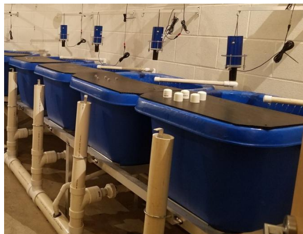
Figure 1. Experimental system consisting of 190-liter tanks with partial (~50%) overhead covers and randomly assigned treatments of half-round pipe array, spherical array, or control (no enrichment).
