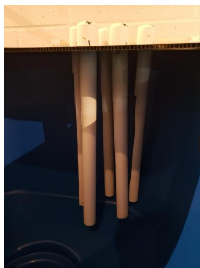
Figure 2. Pipe enrichment array consisting of 40.6 cm tall, 3.2 cm outside diameter polyvinyl chloride pipe cut in half vertically.
