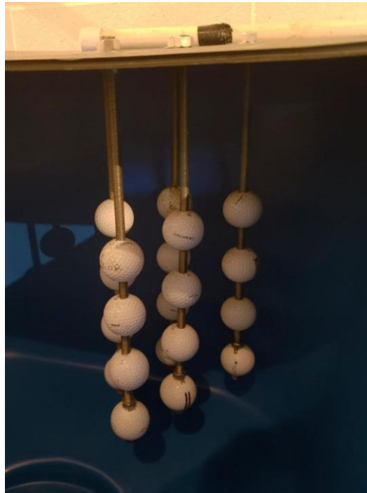
Figure3. Spherical enrichment array consisting of 9.5 mm threaded rods with six 4.3 cm spheres (golf balls) spaced approximately 2.5 cm apart.
