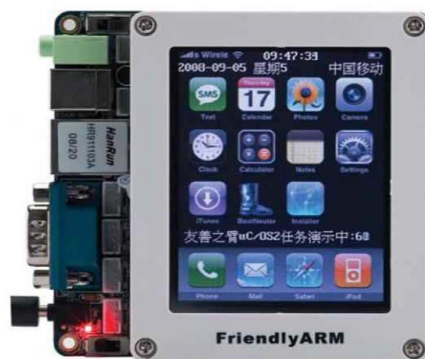
Fig3:ARM9 S3C2440A microcontroller.
