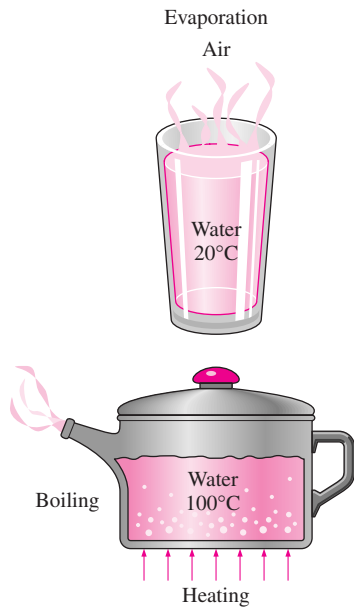
FIGURE 10-1 A liquid-to-vapor phase change process is called evaporation if it occurs at a liquid–vapor interface and boiling if it occurs at a solid–liquid interface.
