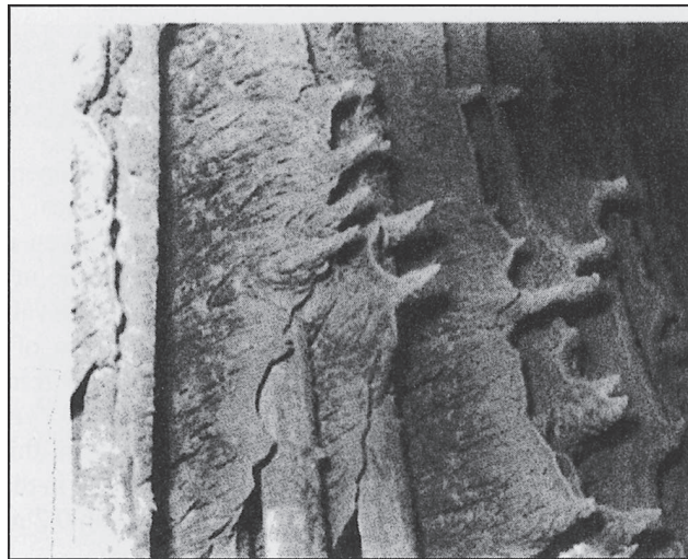
FIGURE 13-9 Precipitation fouling of ash particles on superheater tubes (from Steam, Its Generation, and Use , Babcock and Wilcox Co., 1978).
