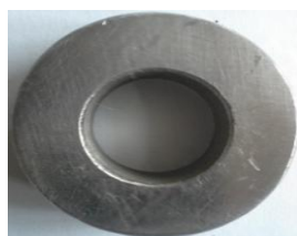
Fig.2 A sample ring specimen
