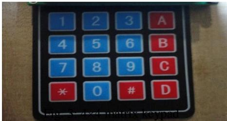
Fig. 2: Keypad of the electronic lock system
