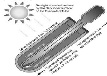
**Fig.6 Evacuated Tube Collector [1]**
