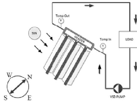
**Fig.8 Diagram of Test Arrangement [5]**
