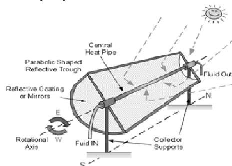
**Fig 7. Concentrating Collector [1]**
