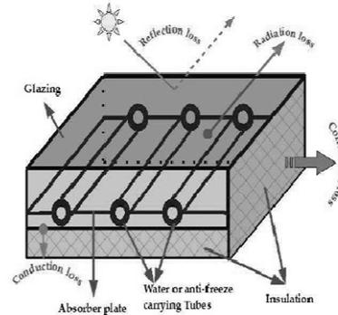
**Fig.5 Flat Plate Collector [1]**
