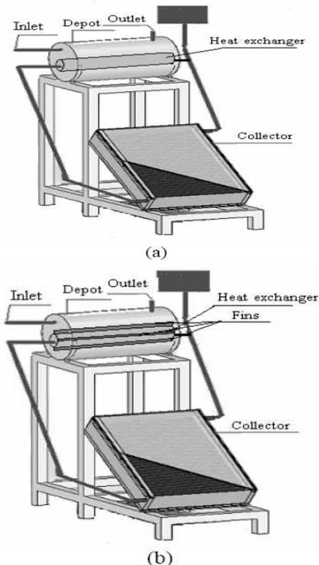
Fig. 9. (a) Classical System (b). Finned System [8]
