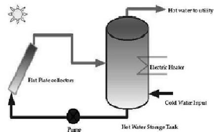
Fig1. Open Loop Active System[1]
