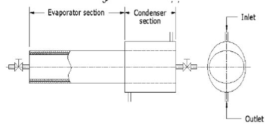
Fig.10. Detail of heat pipe.[9]
