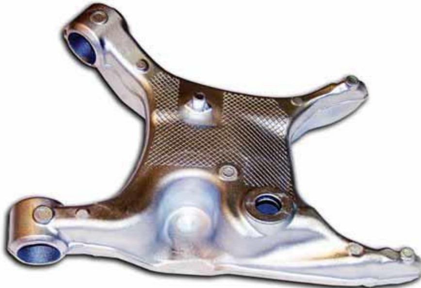
Figure 2 This rear lower control arm for the automotive industry was cast hollow with A356 aluminum alloy through a low-pressure permanent mold casting process [7]
