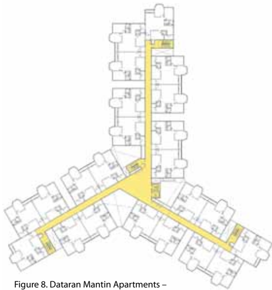
Figure 8. Dataran Mantin Apartments – Double-loaded/central corridors.
