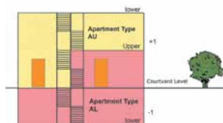
Figure 2. Basic interlocking apartment module.
