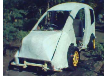
Figure 6: TODS Prototype Vehicle equipped by ESP,4WS & AS
