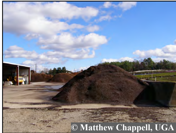
Figure 6.14 Piles of bark, sand, peat, or other substrate components need to be kept on concrete pads until needed to reduce weed seed contamination.
