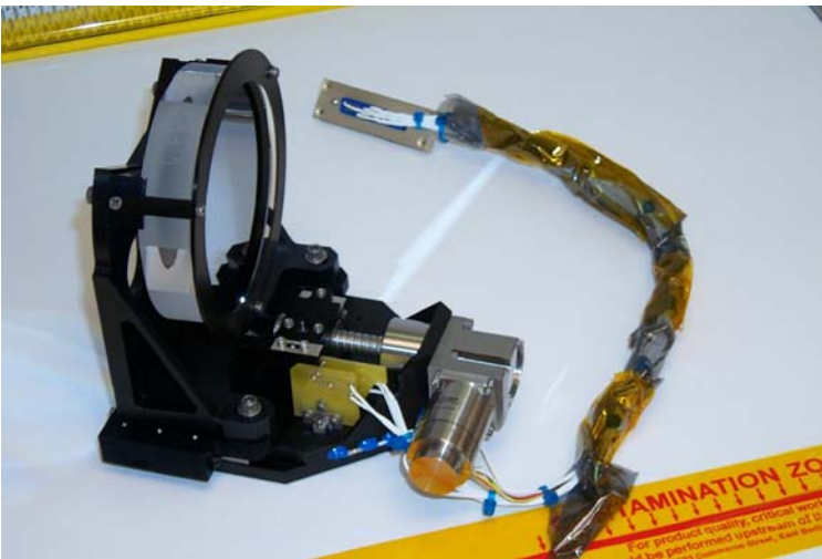
Figure 13 Grating FL-7 in its flight mounting. Two of the four alignment facets on the margin of the grating blank are visible. The focus mechanism includes motor, gearhead, and ball screw. Two small circuit boards hold LEDs and photodiodes for the limit sensors.
