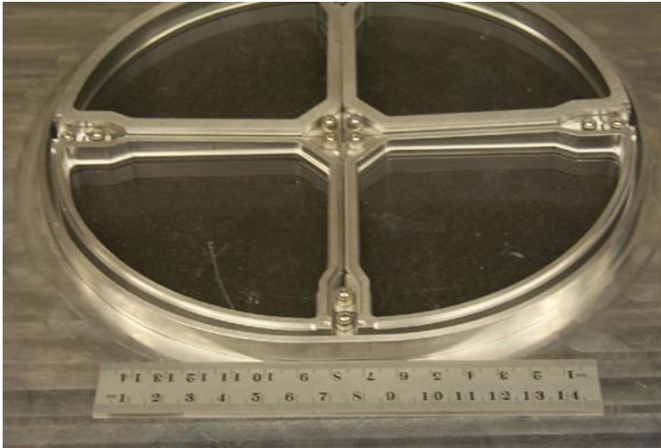
Figure 4 Engineering model of EIS front filter array. Four frames are in place. This view of the array is before the aluminum foils were mounted.
