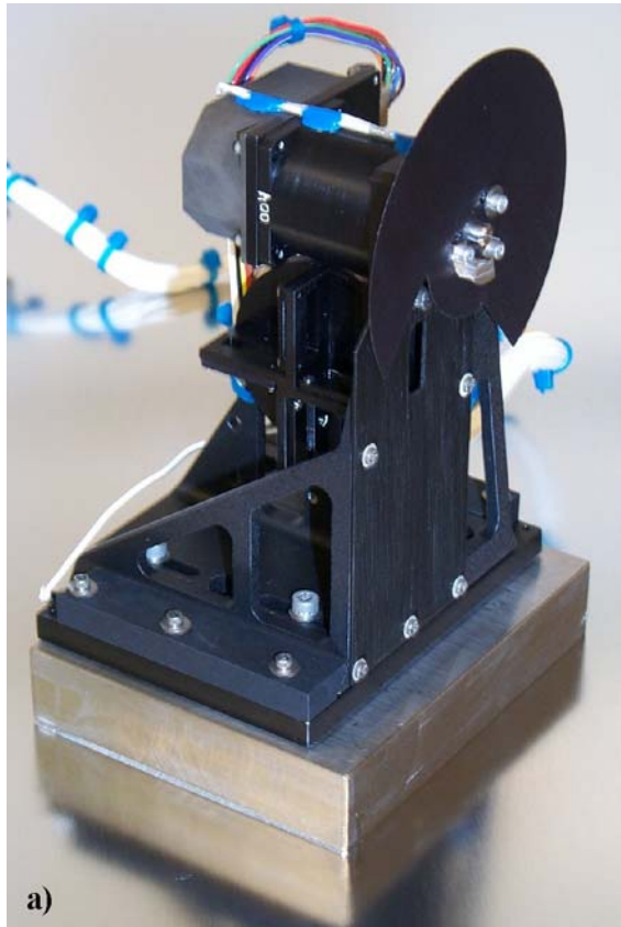
Figure 8 (a) Slit/slot mechanism assembly. The four slits are on a paddle wheel and are exchanged by 90 degree rotations of the wheel. The shutter blade and motor are also attached to this assembly. (b) Paddle wheel and slit frame before blackening.
