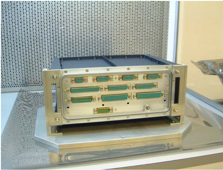
Figure 18 The MHC electronics box is housed in a single enclosure. Boards mounted in the box include the Digital Board (top row of connectors), Analog Board (second row), Auxiliary Board (third row) and the Power Converter Board (bottom connector).
