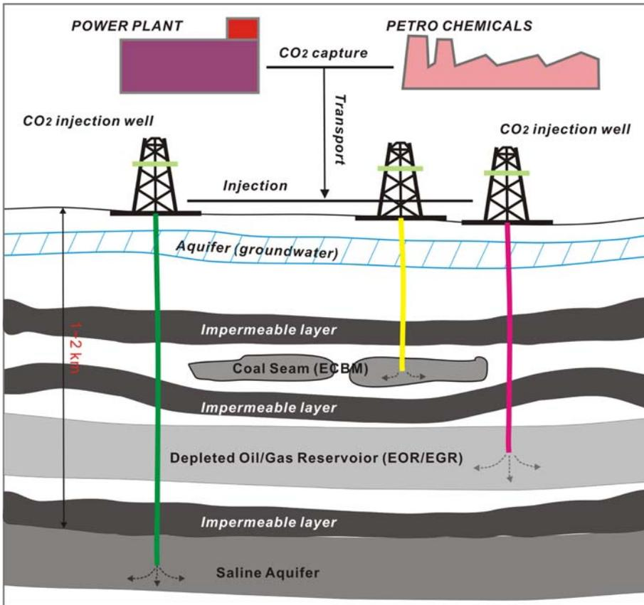
**Fig. 5.** Options of geological storage for carbon dioxide (CO<sub>2</sub>). The figure concept and depth data are from Metz et al. (2005).
