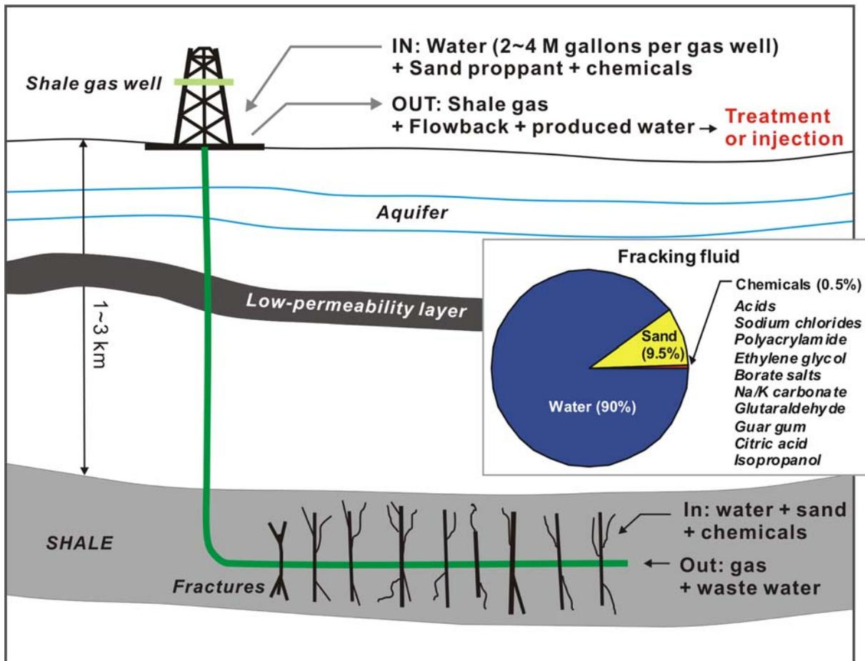
**Fig. 3.** Schematic of hydraulic fracturing (fracking) in shale gas development, also showing the components of the fracking fluid. The figure is modified from IEA (2011).
