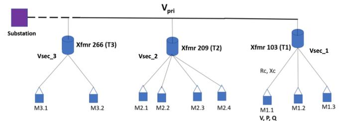
Fig. 4. Network connectivity between Transformers (Xfmrs) 103, 209, 266
