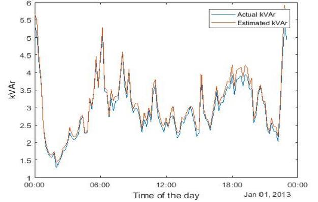
Fig. 5. Estimated vs Actual reactive power profile for transformer 103
