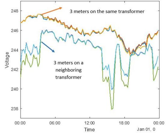
Fig. 2. Voltage profiles of neighboring and non-neighboring meters
