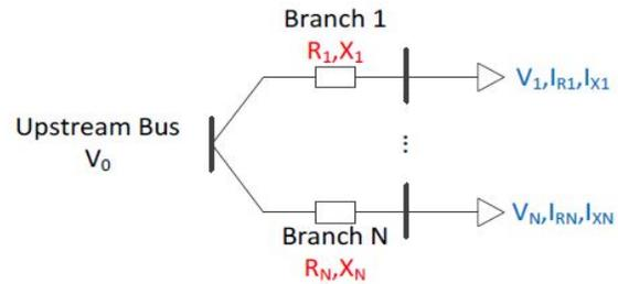
Fig. 3. Radial distribution system secondary system parameter estimation. The measured values (blue) are used to estimate the circuit topology and impedance (red) [3]
