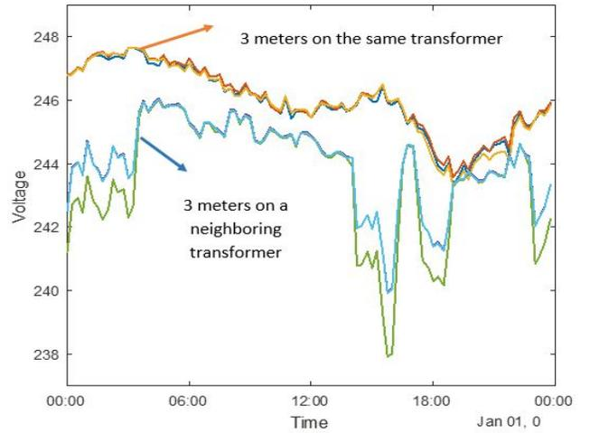
Fig. 4. Voltage profiles of neighboring and non-neighboring meters
