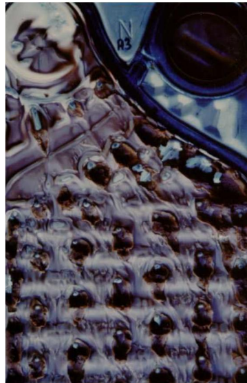
Fig. 2. Reaction Fouling (Protein Deposition) on a Plate and Frame Exchanger Plate
