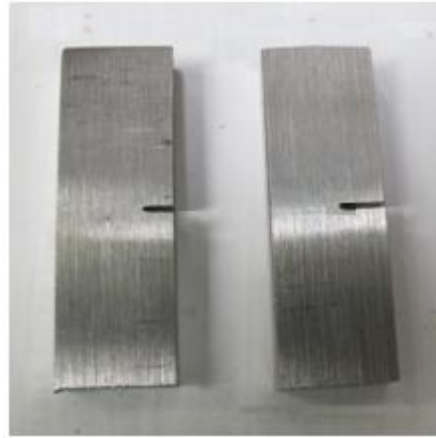
Figure 6. Specimen A1 ( a=0.2W ), A2 ( a=0.4W )
